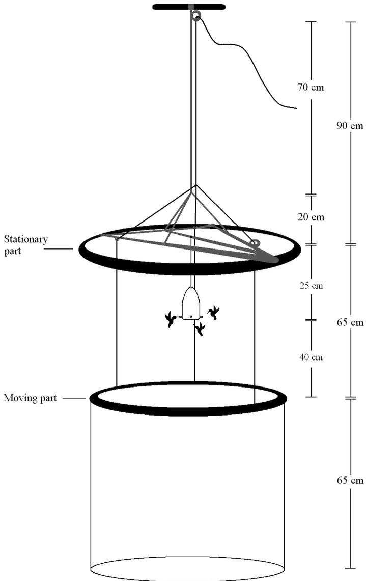
**Figure 1.** Details of the Ruschi net trap, designed for hummingbirds.
